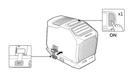
3. Connect the plug and turn the power on
